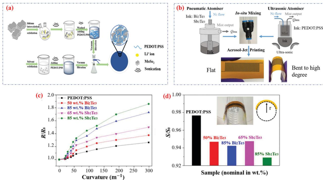
Fig. 6 (a) Schematic illustration of the preparation of the  $\text{MoSe}_2$ /PEDOT:PSS composite; (b) schematic of the *in situ* mixing and aerosol jet printing method; (c and d) flexing test of printed  $\text{Bi}_2\text{Te}_3$  and  $\text{Sb}_2\text{Te}_3$ /PEDOT:PSS nanocomposites. Produced with permission.<sup>100</sup> Copyright © 2017 IOP Publishing Ltd.<sup>156</sup> Copyright © 2018 American Chemical Society.
