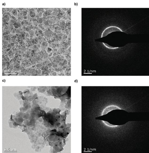
**Fig. 4** (a) EM micrograph of  $1 \text{ mg mL}^{-1}$  P3. (b) EM diffraction pattern of  $1 \text{ mg mL}^{-1}$  P3. (c) Transmission electron microscope image of  $1 \text{ mg mL}^{-1}$  P3. (d) Transmission electron microscope diffraction pattern of  $1 \text{ mg mL}^{-1}$  P4.
