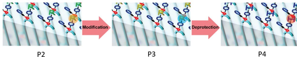
**Scheme 2** Schematic representation of the multi-step reaction, which was conducted “on surface” of the polymer platelets: 1. step: modification of the Br-group to a thioacetate-group. 2. step: cleavage of the 2-acetylthioethyl protective group.
