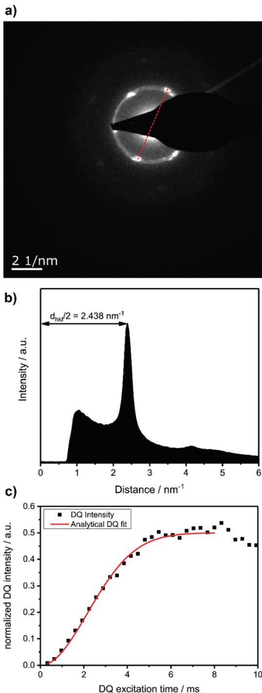
Fig. 1 (a) Diffraction pattern of a single crystal **P1** showing the (110) and (200) plane. (b) Radial intensity profile of the diffraction pattern. (c) Double quantum build-up curve of solution crystallized **P1**, recorded at 25 kHz MAS,  $T = 25\text{ }^{\circ}\text{C}$ , and 202 MHz  $^{31}\text{P}$  Larmor frequency.
