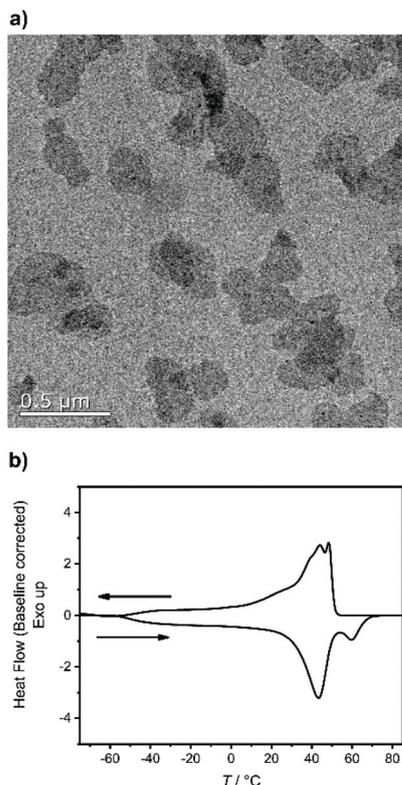
**Fig. 3** (a) Transmission electron microscope micrograph of the single P3 crystals ( $0.1 \text{ mg mL}^{-1}$ ). (b) Differential scanning calorimetry (baseline corrected) of P3 showing the second heating and cooling curve with a  $T_g$  at  $-49 \text{ }^\circ\text{C}$  and  $T_m$  at  $58 \text{ }^\circ\text{C}$  determined in the second heating curve.
