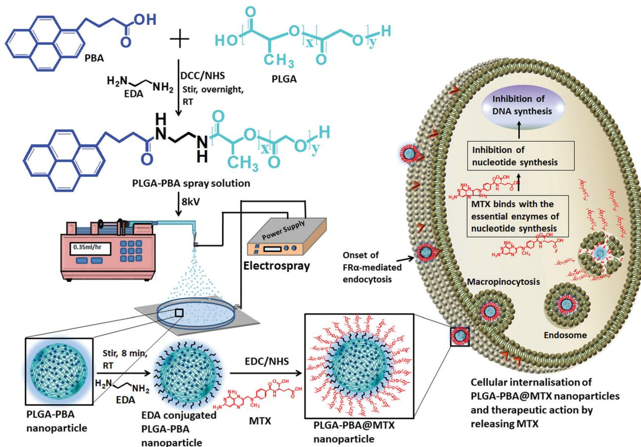
**Scheme 1** Schematic representation of the PLGA–PBA nanoparticle synthesis from the PBA-modified PLGA polymer and the subsequent preparation of PLGA–PBA@MTX nanoparticles to demonstrate the therapeutic action by releasing MTX after intracellular delivery.
