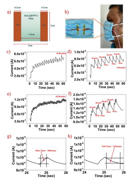
Fig. 6 (a) Schematic of a breath sensor. (b) Integration of the sensor in the breath mask. (c) Continuous-time response of SnS<sub>2</sub> QD/PVA under normal breath. (d and e) Slow and fast breath patterns over a period of 60 seconds. (f) Three breath iterative breathing patterns for five cycles. (g and h) The rise time and fall time of the fabricated sensor were  $\sim 300$  ms and  $\sim 710$  ms.
