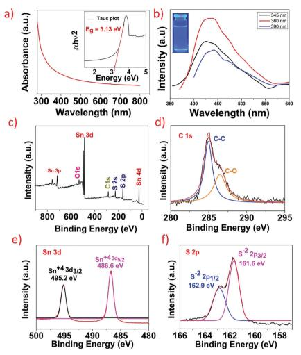
Fig. 3 (a) UV-Visible absorption spectra of  $SnS_2$  QDs; the inset is the Tauc plot showing a bandgap of  $\sim 3.13$  eV. (b) Photoluminescence spectra of  $SnS_2$  QDs at different excitation from 345 nm to 390 nm. (c) XPS survey spectra of  $SnS_2$  QDs. (d) High resolution spectra of C 1s. (e) High resolution spectra of Sn 3d. (f) High resolution spectra of Sp.
