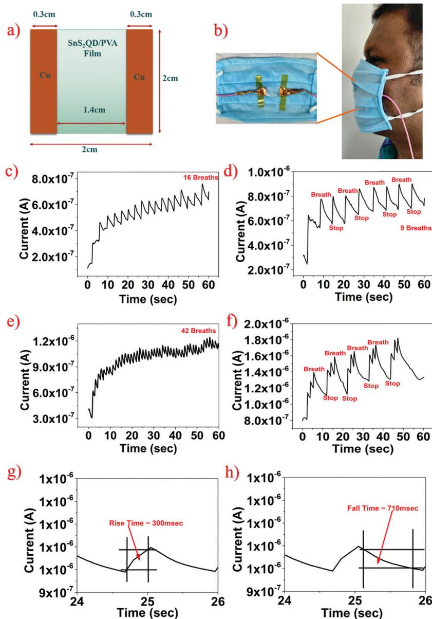
Fig. 6 (a) Schematic of a breath sensor. (b) Integration of the sensor in the breath mask. (c) Continuous-time response of SnS<sub>2</sub> QD/PVA under normal breath. (d and e) Slow and fast breath patterns over a period of 60 seconds. (f) Three breath iterative breathing patterns for five cycles. (g and h) The rise time and fall time of the fabricated sensor were  $\sim 300$  ms and  $\sim 710$  ms.
