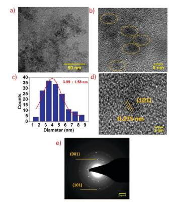
Fig. 2 (a and b) TEM image of the synthesized SnS<sub>2</sub> QDs, (c) size distribution of SnS2 QDs, calculated average diameter of SnS2 QDs is  $3.99 \pm 1.58$  nm, (d) HRTEM lattice fringes of SnS<sub>2</sub> QDs, and (e) SAED pattern of SnS<sub>2</sub> QDs.
