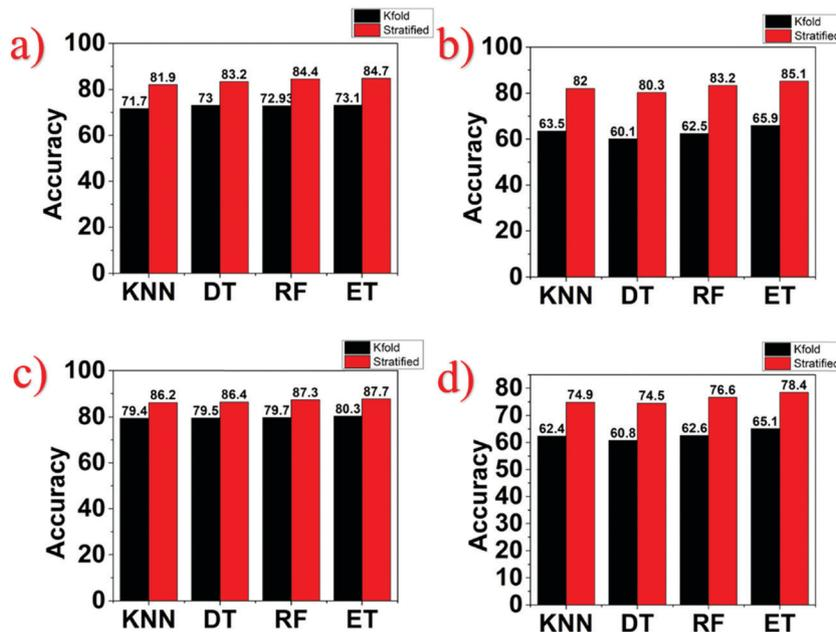
Fig. 9 *k*-Fold and repeated stratified *k*-fold validation methods used for the performance evaluation of both binary and multi-class classifications: (a) breath and pressure, (b) breath and strain, (c) pressure and strain and (d) breath, pressure, and strain respectively.
