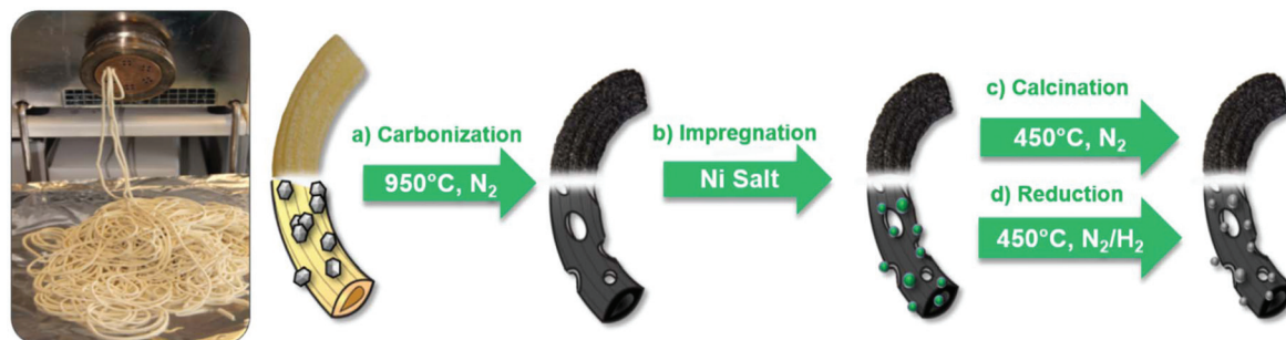
Fig. 3 Schematic representation of the catalyst synthesis protocol starting from the extrusion, carbonization, calcination, and reduction steps.
