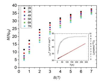
Fig. 6 Field dependence of the magnetisation (M) measured in the T = 2-7 K and B=0.5-7.0 T temperature and field ranges. The inset shows the plot of  $\chi_M T$  vs. T ( $\circ$ ) in the range T = 5-300 K and B = 0.1 T, and the  $1/\chi_{\rm M}$  vs. T ( $\square$ ) data. The solid line is a fit of the experimental data to the Curie-Weiss law.
