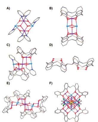
Fig. 1 Single crystal X-ray structures of 1 (A), 2 (B), 3 (C), H<sub>8</sub>L1 (D), 4 (E) and 5 (F). Colour code C - grey, O - red, N - royal blue, Mn<sup>II</sup> - pale blue, Mn<sup>III</sup> - purple, Cl - green, H - white. Hydrogen atoms (except those involved in lower-rim H-bonding in D), <sup>t</sup>Bu groups, ligated solvent molecules and co-crystallised solvent/anions omitted for clarity.
