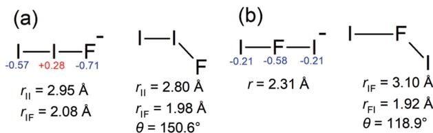
Fig. 4 Calculated equilibrium geometries at the CCSD(T)//def2-TZVPD level of theory for: (a) [I-I-F]<sup>-</sup> and [I-I-F], and (b) [I-F-I]<sup>-</sup> and [I-F-I]. NBO charges (red and blue font) are given for the anions. The lowest energy isomer, [I-I-F]<sup>-</sup> has C<sub>∞h</sub> symmetry, and [I-I-F] has C<sub>s</sub> symmetry.
