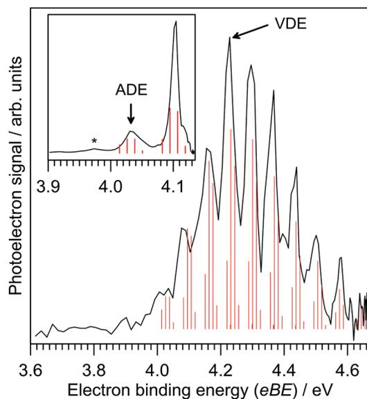
Fig. 1 Photoelectron spectra for IF<sub>2</sub><sup>−</sup> at  $h\nu = 4.66$  eV and 4.13 eV (inset) and Franck–Condon simulation (red sticks) of the D<sub>0</sub> ← S<sub>0</sub> detaching transition for the [F–I–F]<sup>−</sup> isomer. Electron binding energy (eBE) and electron kinetic energy (eKE) are related by  $eBE = h\nu - eKE$ , where  $h\nu$  is the photon energy.
