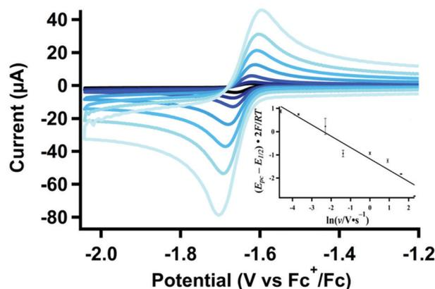
Fig. 1 Variable scan-rate CVs (0.025–10 V s<sup>-1</sup>) of [Pt(depe)<sub>2</sub>](PF<sub>6</sub>)<sub>2</sub> (**1**) (1.06 mM) with CH<sub>2</sub>(TBD)<sub>2</sub>-HPF<sub>6</sub> (5.00 mM) and (b) linear plot for the change in cathodic peak potential used for calculating *k*<sub>obs,H<sup>+</sup></sub>. Additional data used for calculation shown in Fig. S1 and S2 (ESI†).
