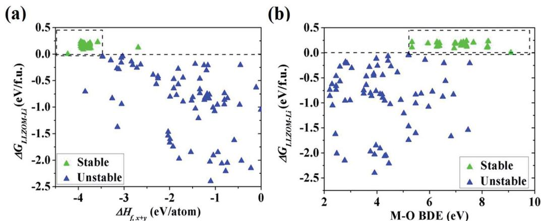
Fig. 5 The dependence of the reaction energy  $\Delta G_{\text{LLZOM-Li}}$  of Li|LLZOM interface on (a)  $\Delta H_{f,x+y}$  and (b) M–O bond dissociation energy. The dotted boxes represent the most appropriate range for each feature.
