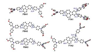
Fig. 2 The DFT-optimized geometrical structure of the studied HTMs.
