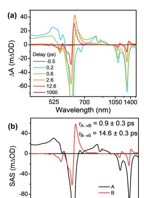
Fig. 6 (a) fsTA spectra and (b) species-associated spectra (SAS) of Bn-TTz++ in CH<sub>3</sub>CN excited at 620 nm ((A)  $^2*TTz^+$ + (D<sub>n</sub>), (B)  $^2*TTz^+$ + (D<sub>1</sub>)). The wavelength axis is plotted in reciprocal space. Time constants are for the representative data set shown here; averages and standard deviations from multiple experiments are given in Table 1.
