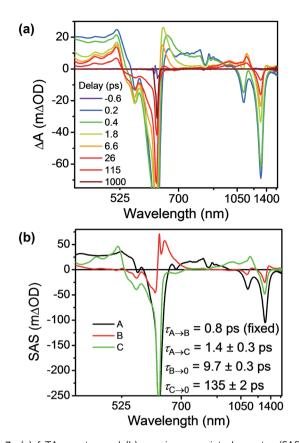
Fig. 7 (a) fsTA spectra and (b) species-associated spectra (SAS) of TTzExVBox  $^{3+*}$  in CH $_3$ CN excited at 620 nm ((A)  $^{2*}$ TTz $^{+*}$  (D $_1$ ), (B)  $^{2*}$ TTz $^{+*}$  (D $_1$ ), (C) TTz $^{2+}$ -ExV $^{+*}$ ). The wavelength axis is plotted in reciprocal space. Time constants are for the representative data set shown here; averages and standard deviations from multiple experiments are given in Table 1.
