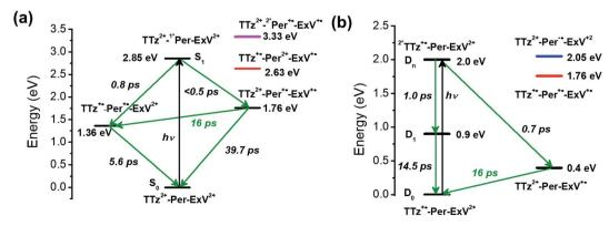
Fig. 5 Energy level diagrams of (a)  $Per \subset TTzExVBox^{4+}$  and (b)  $Per \subset TTzExVBox^{3++}$  in  $CH_3CN$ , in which the zero energy level is taken to be the  $Per S_0$  state in (a) and the  $TTz^{++} D_0$  state in (b), respectively. The ICT pathways from  $ExV^{++}$  to  $TTz^{2+}$  as well as the corresponding timescales are highlighted in red. The states involved in superexchange mixing are shown in red, blue, and magenta.
