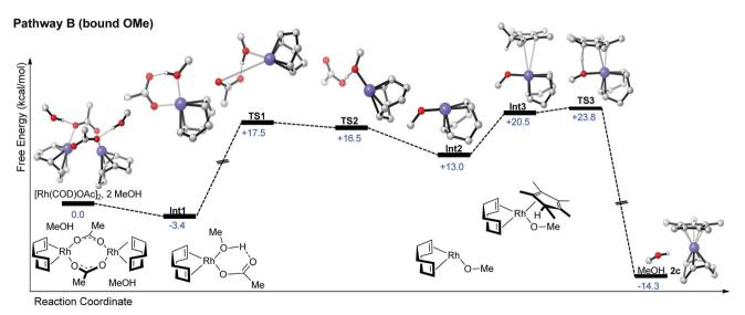
Scheme 2 Potential reaction profiles proceeding form the [Rh(COD)OAc]<sub>2</sub> to RhCp\*(COD). Each of the reaction pathways is characterized by roughly similar energetic profiles. Computations at the PBE0-dDsC/TZ2P//M06/def2-SVP level (see ESI for details†).
