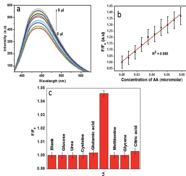
Fig. 7 (a) Fluorescence restoration of CD- $\text{Fe}^{3+}$  system via the addition of ascorbic acid. (b) Relative fluorescence response of CDs- $\text{Fe}^{3+}$  system ( $F/F_0$ ) with different concentrations of AA, (c) fluorescence response of CDs- $\text{Fe}^{3+}$  system in presence of various biomolecules.
