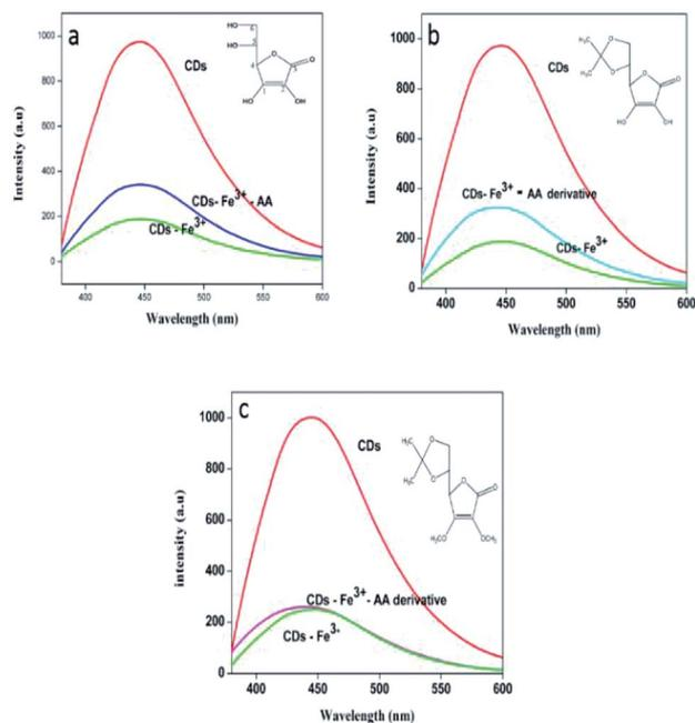
**Fig. 9** (a) PL response of the system with AA, (b) PL response of the system with derivative 8(b), (c) PL response of the system with derivative 8(c). Inset shows the structures of ascorbic acid and their derivatives.
