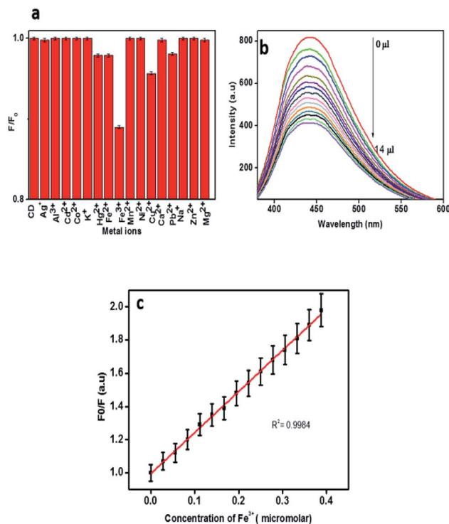
Fig. 6 (a). Fluorescence intensity of CDs in the presence of different metal ions. (b) Steady decline in fluorescence intensity of CDs with increasing  $\text{Fe}^{3+}$  concentration, (c) relative fluorescence response of CDs ( $F_0/F$ ) as a function of  $\text{Fe}^{3+}$  concentration.
