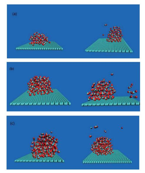
Fig. 2 Snapshot of bubbles under different systems. (a), (b) and (c) are bubbles formed by a system containing 60, 120 and 180  $CO_2$  molecules respectively, the left side is a bubble without an external electric field, and the right side is a bubble under an external electric field.
