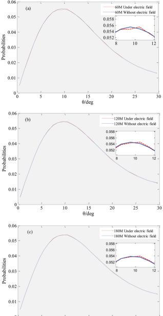
Fig. 5 Distribution of the hydrogen bond angle. (a), (b) and (c) show the hydrogen bond angular distribution of systems with 60, 120, and 180 gas molecules, respectively, under an external electric field (red dashed line) and without an external electric field (blue solid line).
