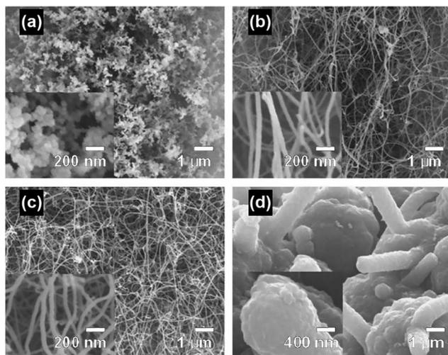
Fig. 5 CNTs synthesized on activated carbon fiber cloth using microwave radiation for (a) 30 s, (b) 60 s, (c) 90 s and (d) 120 s. Reproduced from ref. 38, with permission from Elsevier, 2006.
