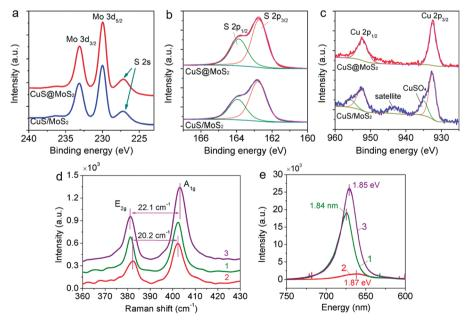
Fig. 2 Spectroscopic characterization. (a-c) XPS spectra of (a) Mo 3d, (b) S 2p and (c) Cu 2p for the Cu<sub>x</sub>S@MoS<sub>2</sub> heterostructures and conventional MoS<sub>2</sub> monolayer transferred onto Cu<sub>x</sub>S nanocrystals. (d) Raman and (e) photoluminescence spectra of (1) monolayer MoS<sub>2</sub> inside the dotted lines in Fig. 1c, (2) conventional MoS<sub>2</sub> monolayer transferred onto Cu<sub>x</sub>S nanocrystals and (3) Cu<sub>x</sub>S@MoS<sub>2</sub> heterostructures
