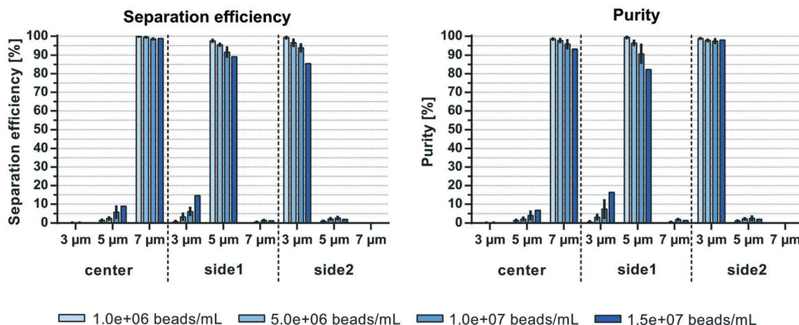
Fig. 5 Particle separation vs. sample bead concentration. Acoustophoretic separation of an equal mixture of  $3$ ,  $5$  and  $7 \mu\text{m}$  polystyrene beads was performed at  $500 \mu\text{L min}^{-1}$  sample flow while altering the initial sample concentrations. Shown are the separation efficiency and purity of the different beads in the three outlets ( $n = 3$ , mean  $\pm$  SD).
