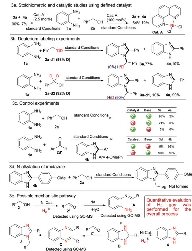
**Scheme 3** Preliminary mechanistic studies and control experiments. **1a** (0.10 mmol) and **2a-d1/2a-d2** (0.20 mmol) were used (see ESI†).
