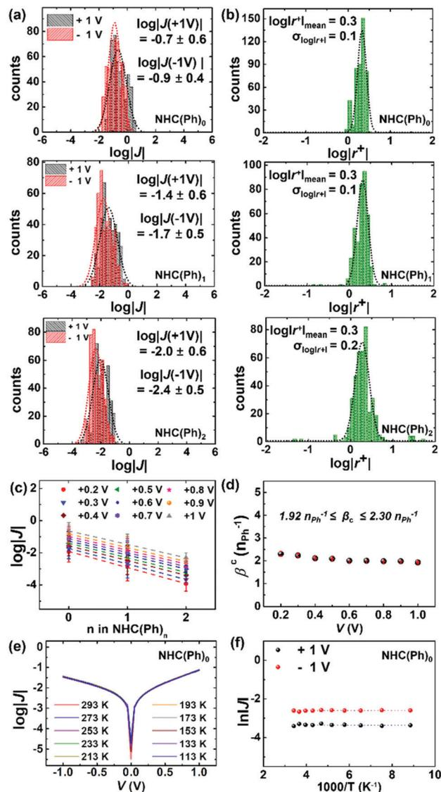
Fig. 2 Histograms of (a)  $\log|J|$  and (b)  $\log|r^{\pm}|$  at  $\pm 1.0$  V for NHC(Ph)<sub>*n*</sub> (*n* = 0, 1, and 2) SAM. (c) Linear correlation between the  $\log|J|$  and the molecular length. (d) Constant  $\beta^c$  value regardless of applied voltage. (e) Exemplary  $\log|J|$ – $V$  traces measured at low temperatures (from 113 to 293 K) for Au<sup>TS</sup>/NHC(Ph)<sub>*n*</sub>//Ga<sub>2</sub>O<sub>3</sub>/EGaIn junctions. (f) The corresponding Arrhenius plots.
