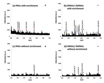
Fig. 3 Real sample SALDI-TOF-MS spectra with (a and b) and without (c and d) enrichment using  $Fe_3O_4$ @COFs ((a1) acenaphthylene; (a2) biphenyl; (a3) phenanthrene; (a4) pyrene; (b1) 1-nitronaphthalene; (b2) 3-nitrodibenzofuran; (b3) 9-nitroanthracene; (b4) 7-nitrobenz[a]anthracene; (c1) 2-hydroxynaphthalene; (c2) 2-hydroxyphenanthrene; (c3) 4-hydroxybiphenyl; (c4) 3-hydroxyfluorene).
