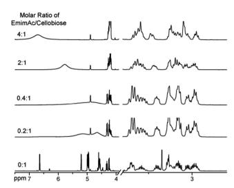
Fig. 4 Effects of different ratios of [Emim][OAc]/cellobiose on the nuclear magnetic peak in the <sup>1</sup>H NMR spectra of cellobiose.<sup>49</sup> Reproduced from ref. 49 with permission from the PCCP Owner Societies.
