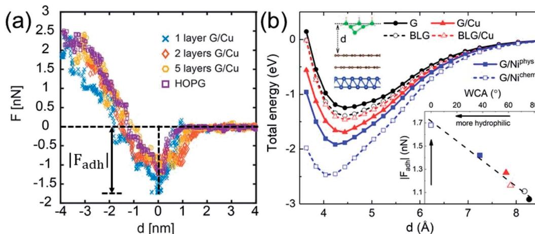
Fig. 5 (a) Measured AFM force profiles for Cu-supported monolayer and multilayer graphene. (b) DFT-simulated AFM energy profiles for free-standing monolayer graphene (G) and bilayer graphene (BLG), Cu-supported monolayer graphene (G/Cu) and bilayer graphene (BLG/Cu), and Ni-supported graphene at the physisorption (G/Ni<sup>phys</sup>) and chemisorption (G/Ni<sup>chem</sup>) states. The inset shows a correlation between  $|F_{\text{adh}}|$  and WCA (both simulated by DFT).
