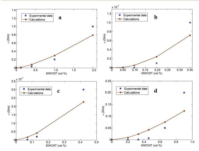
Fig. 2 Experimental results and calculations by the developed model for (a) epoxy/MWCNT,  $^{42}$  (b) PVC/MWCNT,  $^{43}$  (c) epoxy/SWCNT  $^{44}$  and (d) PC/ABS/MWCNT samples.
