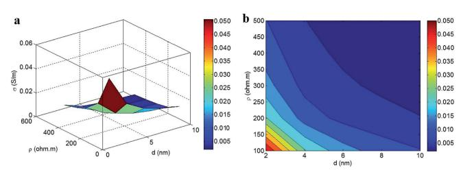
Fig. 6 Expression of conductivity by the developed model at different levels of "d" and " $\rho$ " parameters: (a) 3D and (b) contour plots.
