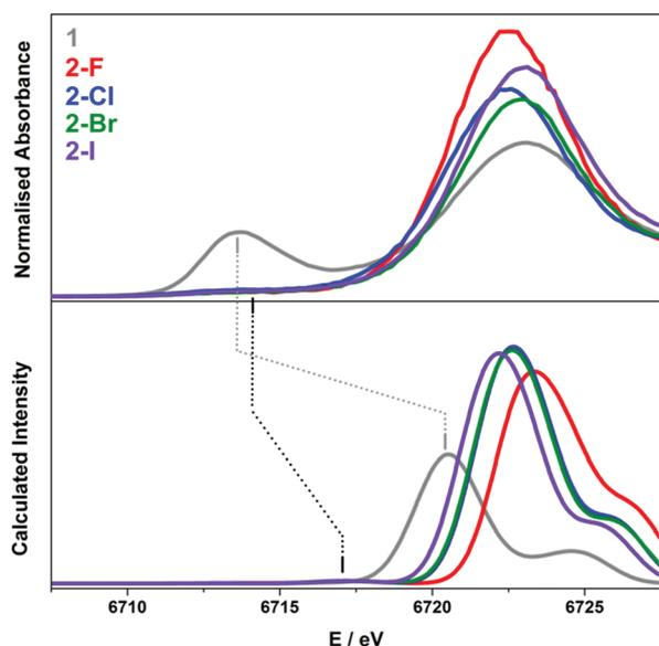
Fig. 7 Comparison of the experimental (top) and calculated (bottom) Sm L<sub>3</sub>-edge spectra of 1 (grey), 2-F (red), 2-Cl (blue), 2-Br (green) and 2-I (violet) obtained from the ZORA-PBE0 TD-DFT calculations. The calculated spectra are shifted +78.6 eV with the intensity in arbitrary units. The grey dashed line links the experimental and calculated Sm(II) white-line peaks; the black dashed line links the experimental and calculated Sm(III)–X pre-edge peaks.
