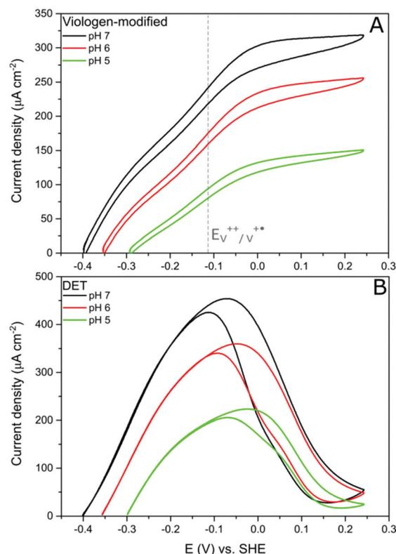
Fig. 7 Comparison of cyclic voltammograms of *DdHydAB* immobilized on viologen-modified GCE (A) and in a DET system on a PGE (B) at three different pH values in an aqueous buffer. Conditions:  $5$  mV  $s^{-1}$ ,  $25$  °C,  $1000$  rpm,  $100\%$   $H_2$ .
