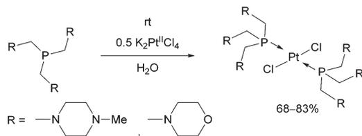
**Scheme 11** Reaction of tris(aminomethyl)phosphines with  $\text{K}_2\text{Pt}^{\text{II}}\text{Cl}_4$ .
