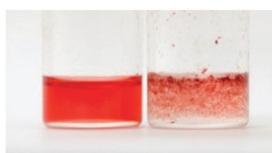
Fig. 10 Photograph of Cyt. c (3 mg mL -1 ) mixed with [C 4 mim][Tf 2 N] (right), and [C 4 mim][Tf 2 N]/ 7 /water mixture (left).
