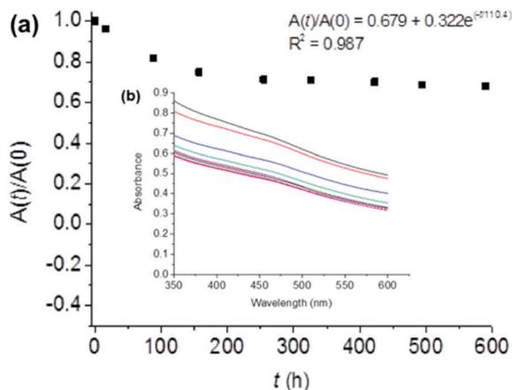
Fig. 3 Stability of BP flakes in solution. (a) The degradation of FL-BP flakes in aqueous 1% w/v Z7950 determined by the ratio of optical absorption at 465 nm at time  $t$  and time zero. The observed lifetime from the fitted decay is around 110 h, whilst ca. 68% of the flakes remains undegraded over a period of ca. 1 month in this media. Inset: Data fitting and  $R^2$ . (b) UV-Vis absorption data used to construct the plot in (a).
