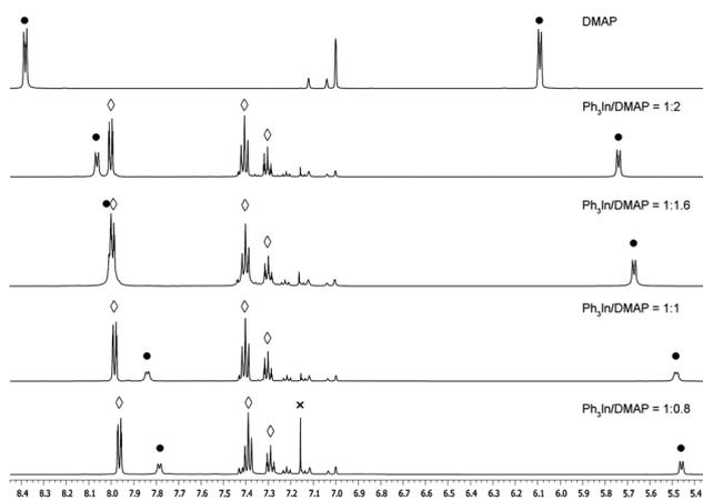
Fig. 1 Ph<sub>3</sub>In(DMAP) stoichiometry experiments. ● DMAP. ◇ Ph<sub>3</sub>In. × Benzene (resulting from Ph<sub>3</sub>In decomposition).
