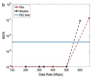
Fig. 2 Top: Plot of electrical power vs. frequency of BBEHBO-PPV films and solution. The dotted line shows the reference -3 dB bandwidth point. The frequency response of commercial phosphor plate (CL-840) is also shown for comparison. Bottom: Bit Error Rate (BER) vs. data rate using PAM-2 of BBEHBO-PPV films and solution.
