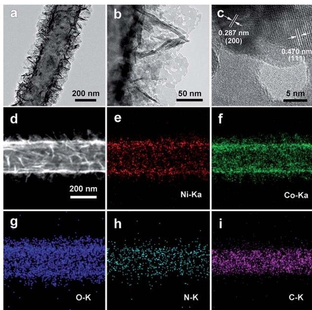
Fig. 3 (a, b) Typical TEM images of  $\text{NiCo}_2\text{O}_4$  nanosheets on carbon nanofiber films at different magnifications; (c) an HRTEM image of  $\text{NiCo}_2\text{O}_4$  nanosheets; (d–i) HAADF-STEM and corresponding EDX elemental mappings (Ni, Co, O, N, C) of  $\text{NiCo}_2\text{O}_4$ @CNFs.
