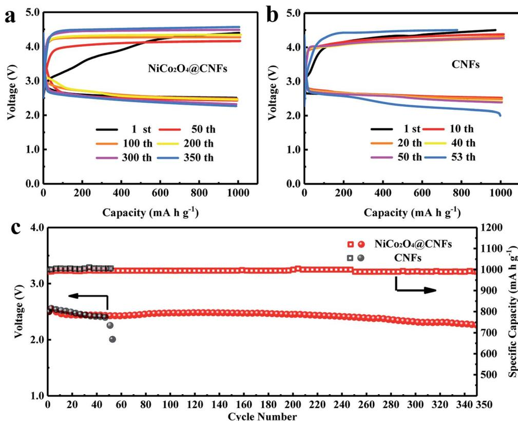
Fig. 5 (a and b) The cycling performance of  $\text{NiCo}_2\text{O}_4@\text{CNFs}$  and CNFs cathodes at a current density of  $200 \text{ mA g}^{-1}$  and a specific capacity limit of  $1000 \text{ mA h g}^{-1}$ ; (c) the terminal discharge voltage as a function of cycle number for Li- $\text{O}_2$  batteries with  $\text{NiCo}_2\text{O}_4@\text{CNFs}$  and CNFs cathodes.
