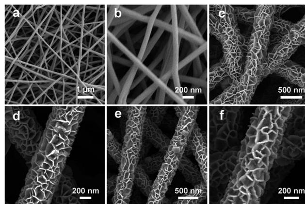
Fig. 2 FESEM images of (a, b) carbon nanofiber films at different magnifications; (c, d) Ni–Co–O precursor nanosheets grown on carbon nanofibers at different magnifications; (e, f) NiCo<sub>2</sub>O<sub>4</sub> nanosheets grown on carbon nanofibers at different magnifications.
