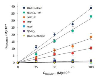
Fig. 3 Variation in equilibrium concentration of CO<sub>2</sub> (C<sub>reacted</sub>) plotted as a function of initial reagent concentration at T = 293 K (repeated in triplicate, analysing 300 images with a range of 4000-7000 plugs of  $CO_2$ ).
