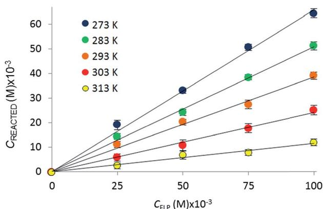
Fig. 4 Variation in the equilibrium concentration of captured CO<sub>2</sub>, plotted as a function of initial FLP (B(C<sub>6</sub>F<sub>5</sub>)<sub>3</sub> and *t*Bu<sub>3</sub>P) concentration at  $T = 273$  K, 283 K, 293 K, 303 K, and 313 K (repeated in triplicate analysing 300 images with a range of 4000–7000 plugs of CO<sub>2</sub>) (see ESI† for plots for the other systems).
