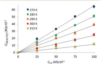
Fig. 4 Variation in the equilibrium concentration of captured  $CO_2$ , plotted as a function of initial FLP (B( $C_6F_5$ )<sub>3</sub> and tBu<sub>3</sub>P) concentration at T=273 K, 283 K, 293 K, 303 K, and 313 K (repeated in triplicate analysing 300 images with a range of 4000–7000 plugs of  $CO_2$ ) (see ESI† for plots for the other systems).
