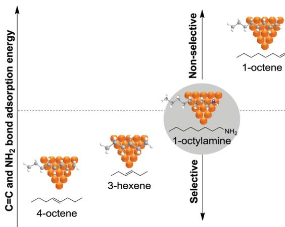
Fig. 32 Correlation between C=C and NH<sub>2</sub> adsorption energy at the surface of a Pt cluster and the selectivity to the corresponding alkenes.
