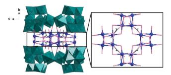
Fig. 1 Representation of the polyanion cluster of 1 (left) and the {Cu<sub>16</sub>} core in the cluster (right). The  $\{W_{11}\}$  building units are shown as teal polyhedra, Cu as blue sphere, O and C as rose and grey sticks
