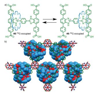
Fig. 27 (a) Pseudo-degenerate molecular shuttle 46 and (b) the MOF formed by reaction of **46** with Zn<sup>II</sup>. Solid state <sup>13</sup>C NMR line shape analysis revealed that the macrocycle continues to shuttle even in the solid state.<sup>64</sup>
