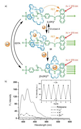
Fig. 14 (a) Metal responsive rotaxane 31 and (b) the observed changes in emission intensity depending on the coordination state.  $^{42}$  The exchange of Zn<sup>II</sup> for Li<sup>I</sup> and *vice versa* was reversible over a number of cycles (inset). Adapted with permission from ref. 42. Copyright 2008 WILEY-VCH Verlag GmbH & Co. KGaA, Weinheim.
