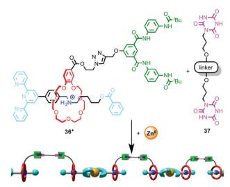
Hierarchical self-assembly of a metallo-supramolecular dimer.<sup>55</sup>
