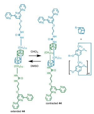
Fig. 25 Solvent responsive monomer 44 that assembles in the presence of Fe<sup>II</sup> to give a stimuli-responsive metallo-supramolecular polymer. 63
