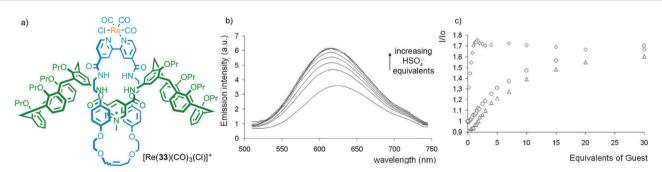
Fig. 16 (a) Beer's hydrogen bonding host  $[Re(33)(CO)_3(CI)]^+$ , (b) its optical read out on  $HSO_4^-$  addition and (c) a comparison with the response of the rotaxane host (diamonds), the corresponding non-interlocked macrocycle (triangles) and an acyclic analogue (circles).<sup>44</sup> Reproduced from ref. 44 with permission from the Royal Society of Chemistry
