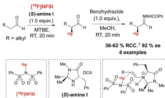
Scheme 5 Chiral imidazolidinone (*S*)-I for the enantioselective  $^{18}\text{F}$ -fluorination of aldehydes with  $^{18}\text{F}$ -NFSI.  $\dagger$ RCC determined by radio-HPLC relative to  $^{18}\text{F}$ -NFSI. DCA = dichloroacetic acid. For  $^{18}\text{F}$ -NFSI, SA = 0.05  $\mu\text{mol}^{-1}$ , ( $n = 3$ ).
