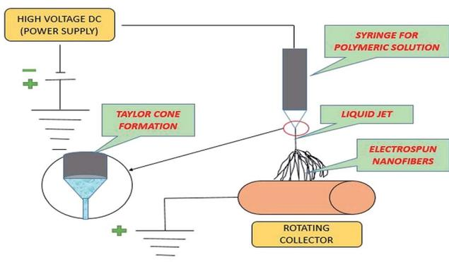
Fig. 6 Diagram shows the formation of Taylor cone in electrospinning technique.<sup>63</sup>
