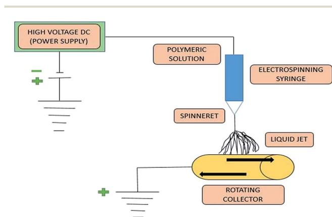
Fig. 1 Schematic block diagram of electrospinning technique.
