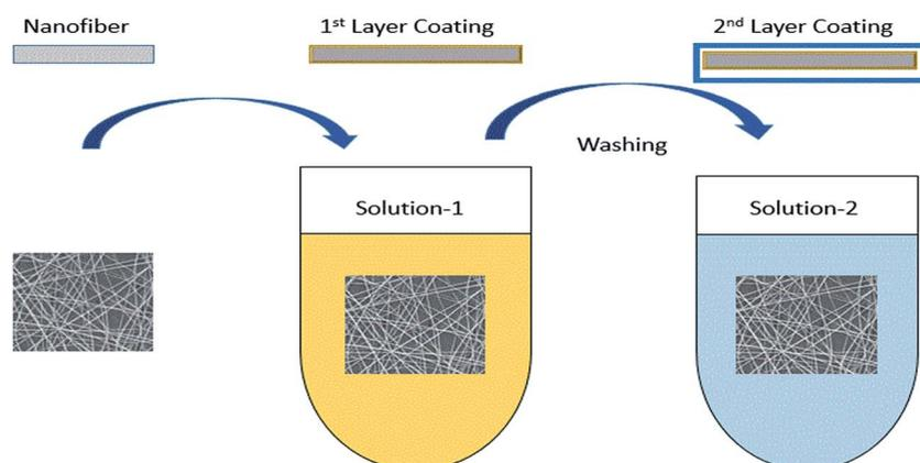
Fig. 9 Layer-by-layer treatment for functionalization of electrospun fibers.
