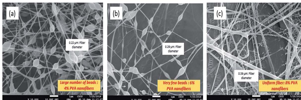
Fig. 8 SEM micrographs of PVA nanofibers indicating the effect of polymer concentration on fiber quality and fiber diameter (a) 4% PVA (b) 6% PVA (c) 8% PVA [ $M_w$ : 146 000–186 000, 99+% hydrolysed, solvent used: deionised water].
