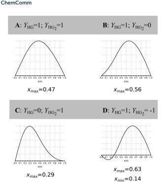
Fig. 2 Simulated Job Plots for various cases of 1:2 stoichiometry with concentration of host =  $0.01\,\text{M}$ ,  $K_1 = 1000\,\text{M}^{-1}$  and  $K_2 = 250\,\text{M}^{-1}$ , i.e. non-cooperative 1:2 binding. Only  $Y_{\text{HG}}$  and  $Y_{\text{HG}_2}$  between cases A–D. The corresponding case for  $Y_{\text{HG}} = 1$  and  $Y_{\text{HG}_2} = 2$  is shown in row 4, column 5 of Fig. 1. Reproduced with permission from ref. 16.
