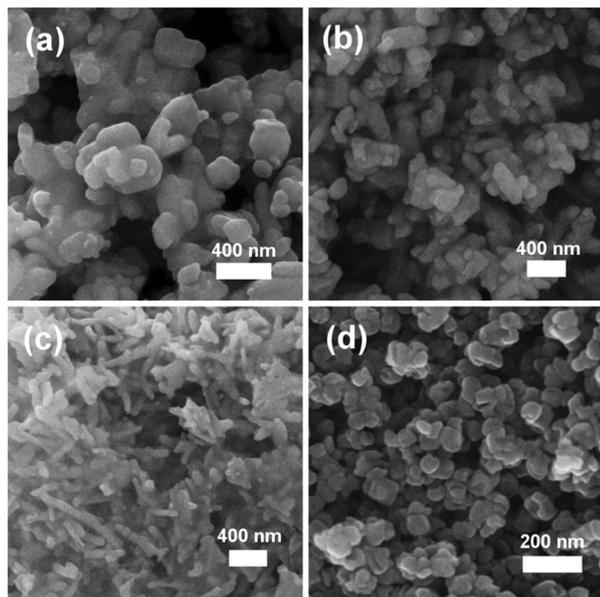
Fig. 3 SEM images of (a)  $\text{LiFePO}_4$ , (b)  $\text{LiFe}_{0.5}\text{Mn}_{0.5}\text{PO}_4$ , (c)  $\text{LiMnPO}_4$  and (d)  $\text{Mn}_3\text{O}_4$  nanostructures prepared from metal alkoxide precursors.
