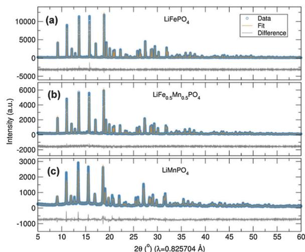
Fig. 2 Rietveld analysis of XRD data of (a)  $\text{LiFePO}_4$ , (b)  $\text{LiFe}_{0.5}\text{Mn}_{0.5}\text{PO}_4$  and (c)  $\text{LiMnPO}_4$  nanostructures prepared from  $[\text{Fe}(\text{O}^t\text{Bu})_2(\text{THF})]_2$ ,  $[\text{Fe}_{0.5}\text{Mn}_{0.5}(\text{O}^t\text{Bu})_2(\text{THF})]_2$  and  $[\text{Mn}(\text{O}^t\text{Bu})_2(\text{THF})]_2$  alkoxides, respectively.
