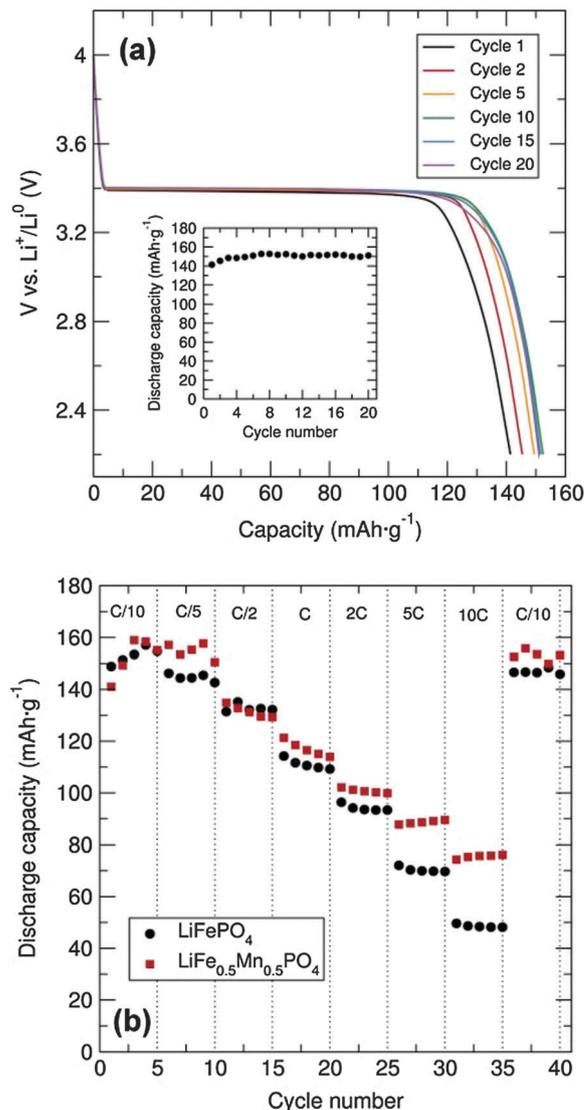
Fig. 4 (a) Cycling performance and capacity fading (inset) of  $\text{C}/\text{LiFePO}_4$  prepared from  $[\text{Fe}(\text{O}^i\text{Bu})_2(\text{THF})_2]_2$  alkoxide precursor (mixed with C black and PTFE in 60 : 30 : 10 weight%) between 2.2 and 4.0 V at C/20 rate. (b) Rate performance of  $\text{C}/\text{LiFePO}_4$  and  $\text{C}/\text{LiFe}_{0.5}\text{Mn}_{0.5}\text{PO}_4$  (mixed with C black and PTFE in 60 : 30 : 10) at different charge–discharge C rates.
