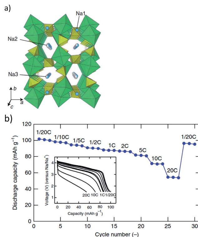
Fig. 8 (a) Na<sub>2</sub>Fe<sub>2</sub>(SO<sub>4</sub>)<sub>3</sub> structure projected along the c axis, and (b) capacity retention upon cycling up to 30 cycles under various rate of C/20 (2 Na in 20 h) to 20 C. Reproduced with permission<sup>80</sup> © 2014, Nature Publishing Group.
