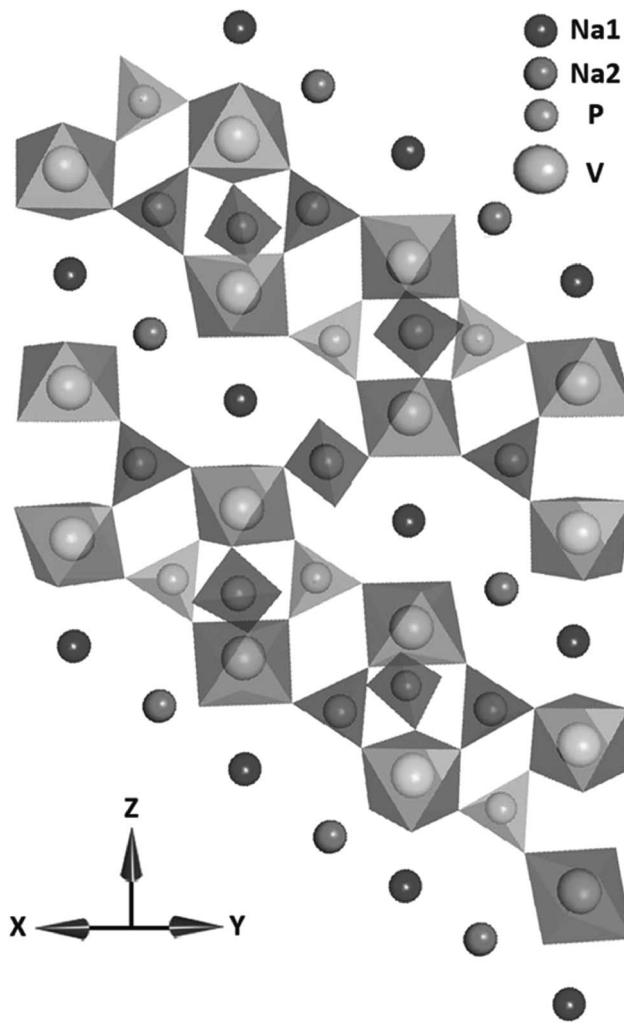
Fig. 9 The crystal structure of  $\text{Na}_3\text{V}_2(\text{PO}_4)_3$  in the  $a$  and  $b$  plane. Reproduced with permission<sup>81</sup> © 2013, WILEY-VCH Verlag GmbH & Co.
