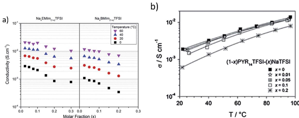
Fig. 18 (a) Isotherms of the conductivity as a function of the molar fraction of  $\text{Na}_x\text{EMIm}_{(1-x)}\text{TFSI}$  and  $\text{Na}_x\text{BMIm}_{(1-x)}\text{TFSI}$  (reproduced with permission<sup>153</sup> © 2014, Elsevier) and (b) ionic conductivity vs. temperature for the  $(1 - x)\text{PYR}_{14}\text{TFSI} - (x)\text{NaTFSI}$  electrolyte. Reproduced with permission<sup>154</sup> © 2014, Elsevier.
