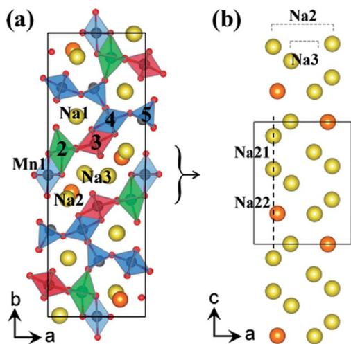
Fig. 5 (a) Crystal structure of  $\text{Na}_{0.44}\text{MnO}_2$  showing Mn and Na binding sites, and (b) the S shaped tunnel configuration along  $c$ -axis with different sodium positions  $\text{Na}_{21}$  and  $\text{Na}_{22}$  in  $\text{Na}_{0.44}\text{MnO}_2$ . Reproduced with permission<sup>35</sup> © 2012, ACS Publications.
