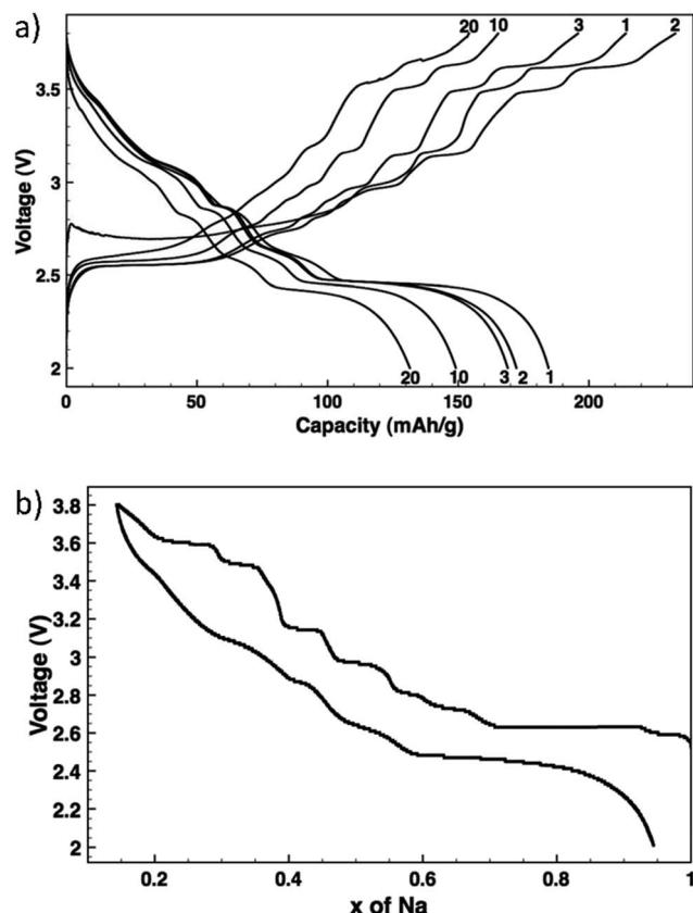
Fig. 4 Voltage profiles: (a)  $\text{Na}_x\text{MnO}_2$  cycled at C/10 with the cycle numbers indicated, and (b)  $\text{Na}_x\text{MnO}_2$  de/sodiation as measured by potentiostatic intermittent titration. Reproduced with permission<sup>36</sup> © 2012, The Electrochemical Society.
