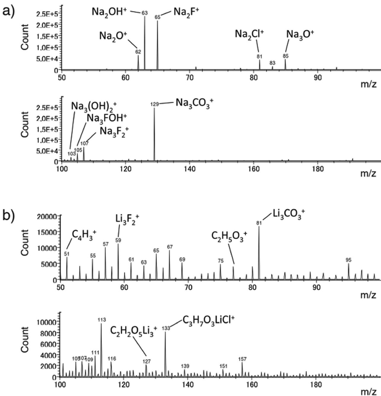
Fig. 21 TOF-SIMS positive ion spectra for the hard-carbon electrodes after the first galvanostatic cycle in (a) sodium and (b) lithium cells. Reproduced with permission<sup>128</sup> © 2011, WILEY-VCH Verlag GmbH & Co.
