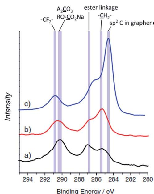
Fig. 20 XPS carbon 1s spectra for the hard-carbon electrodes tested in (a) sodium and (b) lithium cells after the first cycle, and (c) pristine electrode. Reproduced with permission<sup>128</sup> © 2011, WILEY-VCH Verlag GmbH & Co.
