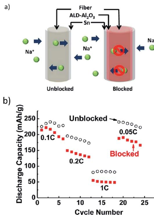
**Fig. 13** (a) Na<sup>+</sup> ions transport along and diffuse through the mesoporous wood fiber structure. Internal transport pathways are blocked by the conformal Al<sub>2</sub>O<sub>3</sub> coating, and (b) the rate performance of the Sn anode deposited on the carbon-coated mesoporous wood fibers. Reproduced with permission<sup>137</sup> © 2013, ACS Publications.
