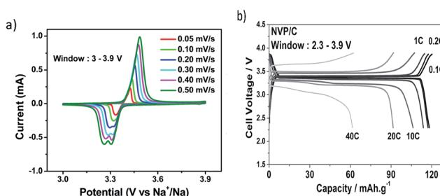
Fig. 10 (a) Cyclic voltammogram of  $\text{Na}_3\text{V}_2(\text{PO}_4)_3$ , and (b) galvanostatic charge and discharge profiles for several C rates. Reproduced with permission<sup>81</sup> © 2013, WILEY-VCH Verlag GmbH & Co.
