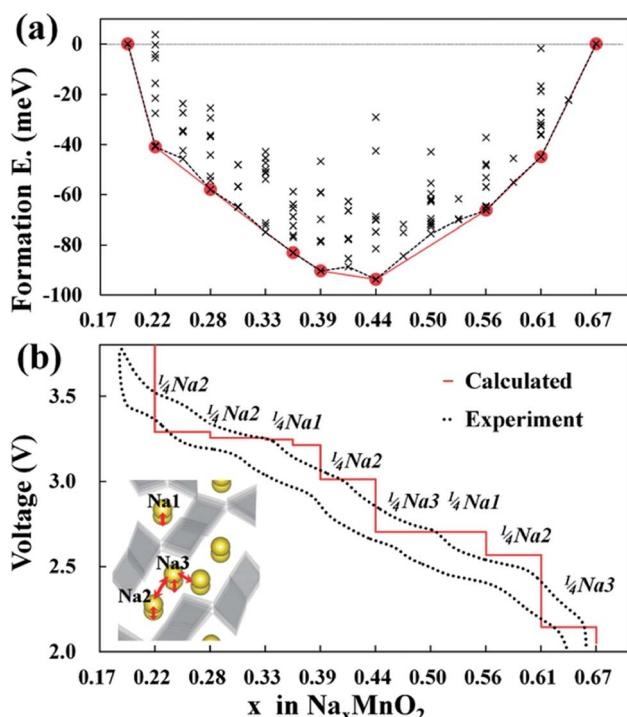
Fig. 6 (a) Formation energies of seven stable intermediate phases during  $\text{Na}_x\text{MnO}_2$  cycling calculated from 156 different sodium configurations, and (b) experimental and calculated voltage profiles for  $\text{Na}_x\text{MnO}_2$  with respect to the minimum energy path of formation energies. Reproduced with permission<sup>35</sup> © 2012, ACS Publications.
