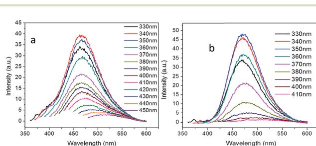
Fig. 4 Excitation-dependent PL emission of the carbon dots passivated with (a) branched PEI (CD<sub>b</sub>) and (b) linear PEI (CD<sub>l</sub>).
