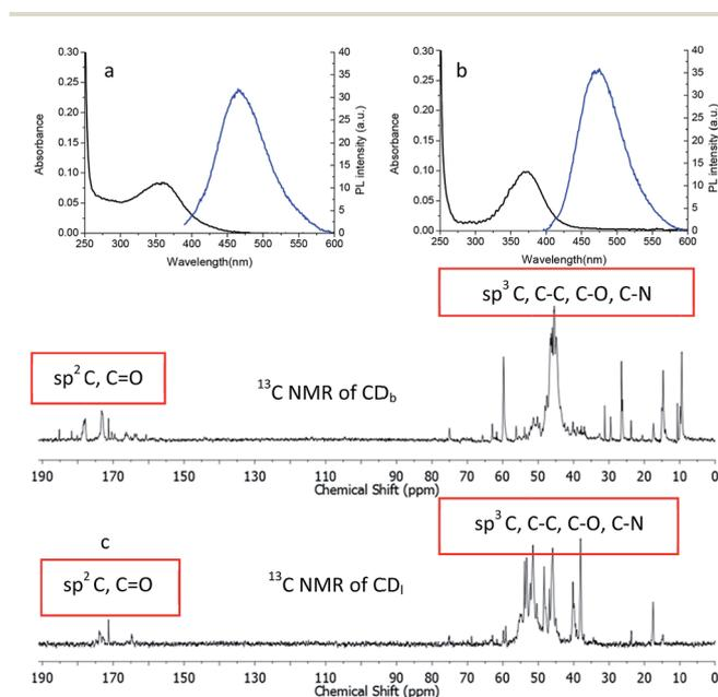
Fig. 3 UV-Vis absorbance and photo luminescent emission spectra (excited at 360 nm) of the carbon dots passivated with (a) branched PEI (CD<sub>b</sub>) and (b) linear PEI (CD<sub>l</sub>). (c) <sup>13</sup>C NMR spectrum of CD<sub>b</sub> and CD<sub>l</sub>.
