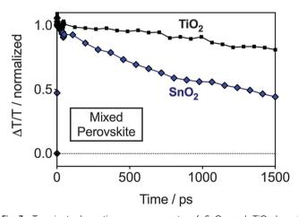
Fig. 3 Transient absorption measurements of  $SnO_2$  and  $TiO_2$ -based planar PSCs. Dynamics of the photo-bleaching bands for photo-excited perovskite measured on a typical working device employing the mixed perovskite (FAPbl<sub>3</sub>)<sub>0.85</sub>(MAPbBr<sub>3</sub>)<sub>0.15</sub> and  $SnO_2$  or  $TiO_2$  as the ESL. The device is held at short circuit condition during the measurement. The probe wavelength is  $\lambda = 750$  nm while pumping at  $\lambda = 520$  nm.
