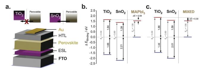
Fig. 1 Energy level diagrams and electron injection characteristics of SnO<sub>2</sub> and TiO<sub>2</sub>-based planar PSCs. (a) Schematic conduction band diagram of the perovskite films and the electron selective layers, TiO2 and SnO2 for (b) MAPbI3 and (c) (FAPbI3)0.85(MAPbBr3)0.15, labeled as 'mixed'
