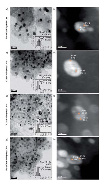
Fig. 5 Bright-field diffraction contrast TEM images with PSDs, Ni atomic percentages determined from parallel-beam EDS (left) and HAADF STEM images with point-mode EDS (right) for catalyst particles taken from 30k-cycled MEAs. (a) and (b) P1-NA, (c) and (d) P2-NA, (e) and (f) P2-SA, (g) and (h) P2-SA-AN. Here  $\sigma$  represents the standard deviation of PSD from at least 100 measurements and the standard deviation of EDS results among 3 different locations.
