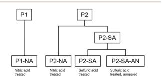
Fig. 1 Schematic showing different catalysts studied in this paper. The precursors were either treated in (1) 1 M nitric acid at 70 °C for 24 h in air (P1-NA and P2-NA) or (2) 0.5 M sulfuric acid at 80 °C for 24 h in nitrogen (P2-SA). After the dealloying, some P2-SA catalysts were thermally annealed at 400  $^{\circ}$ C for 4 h in 5% H<sub>2</sub> and 95% N<sub>2</sub>, marked as P2-SA-AN.
