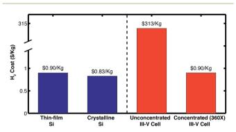
Fig. 7 Comparison of H<sub>2</sub> production costs from devices based on different PV technologies (unconcentrated Si cells in blue, and III-V cells in red). The cost shown for a concentrated cell, is the base  $H_2$  cost and does not include the cost for the concentrator and tracking components.
