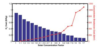
Fig. 6 The bar graph shows the base hydrogen production cost (excluding the cost for solar concentration) as a function of light concentration. The red line shows the breakeven cost for the economically viable implementation of a solar-concentrator and tracking components. (Results are based on a multi-junction thin-film Si PV cell).
