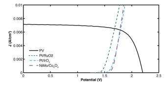
Fig. 2 Current characteristics of various electrolysis components and an 11% a-Si/a-Si/uc-Si PV component. The intersection point between the PV output curve (black solid line) and the different electrolyzers load curves (dotted lines) represents the operational current and voltage of the overall solar-hydrogen generator
