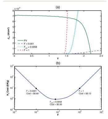
Fig. 3 Top graph shows how the operation of the electrolyzer changes with the geometric factor, F. The bottom figure shows how the cost varies as a function of F.
