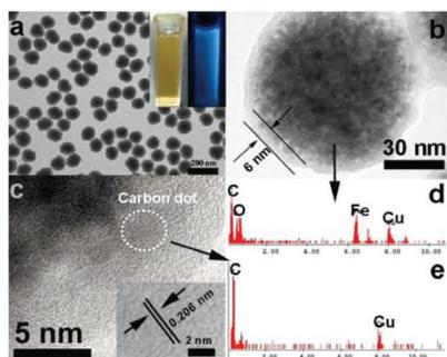
**Fig. 2** (a and b) TEM images of the  $\text{Fe}_3\text{O}_4@\text{C}$ -CDs hybrid NPs. The inset in (a) is the photographs of aqueous dispersions of the hybrid NPs under visible light and UV light (365 nm); (c) High resolution TEM image of the carbon shell. The inset is the lattice fringe of CDs; (d) and (e) Energy dispersive spectrum of the single  $\text{Fe}_3\text{O}_4@\text{C}$ -CDs NP and single CD, respectively.
