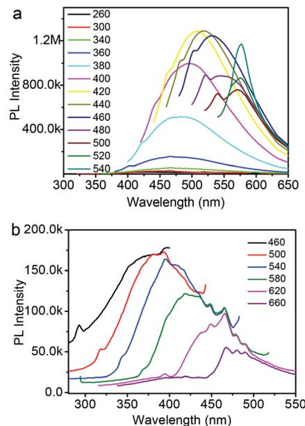
Fig. 4 (a) PL spectra of Fe<sub>3</sub>O<sub>4</sub>@C-CDs NPs obtained with different excitation wavelengths; (b) Upconversion PL spectra of Fe<sub>3</sub>O<sub>4</sub>@C-CDs NPs obtained with different excitation wavelength.
