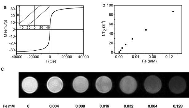
**Fig. 5** (a) The hysteresis loop of  $\text{Fe}_3\text{O}_4\text{@C-CDs}$  NPs measured at room temperature. The left inset shows the respective expanded plots for fields between  $-40$  and  $40$  Oe; (b)  $T_2^*$  relaxation rates as a function of iron concentration (mM) for  $\text{Fe}_3\text{O}_4\text{@C-CDs}$  NPs; (c)  $T_2^*$ -weighted MR images of  $\text{Fe}_3\text{O}_4\text{@C-CDs}$  NPs at different concentrations, corresponding to different amount of Fe.
