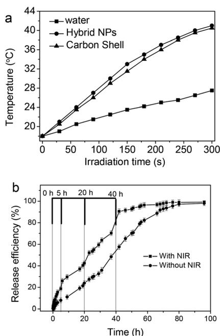
**Fig. 9** (a) The photothermal curves of water,  $\text{Fe}_3\text{O}_4@\text{C-CDs}$  hybrid NPs in water ( $100 \text{ mg L}^{-1}$ ), and corresponding hollow C-CDs carbon shell particles in water under NIR irradiation for 5 min. (b) Release profiles of DOX from the  $\text{Fe}_3\text{O}_4@\text{C-CDs}$  NPs in PBS at  $37 \text{ }^\circ\text{C}$ , irradiated with/without  $1.5 \text{ W cm}^{-2}$  NIR for 5 min at certain time points.
