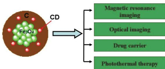
**Fig. 1** Schematic illustration of multifunctional  $\text{Fe}_3\text{O}_4$ @C-CDs hybrid NPs. The magnetic  $\text{Fe}_3\text{O}_4$  nanocrystals and CDs can be used for MRI and fluorescent imaging contrast, respectively. The porous carbon shell embedded with CDs can not only provide high loading capacity for an anti-cancer drug, but also convert the NIR light to heat for combined photothermal/chemotherapy to provide high therapeutic efficacy.
