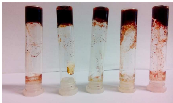
Fig. 6 \text{Cu}(\text{II})\text{:L1} (8 mM/8 mM) Gels in presence of 8mM \text{NaCl} after dissolving L1 in \text{HNO}_3 , \text{H}_2\text{SO}_4 , \text{HBr} , \text{HClO}_4 and p -toluenesulfonic acid (left to right).
