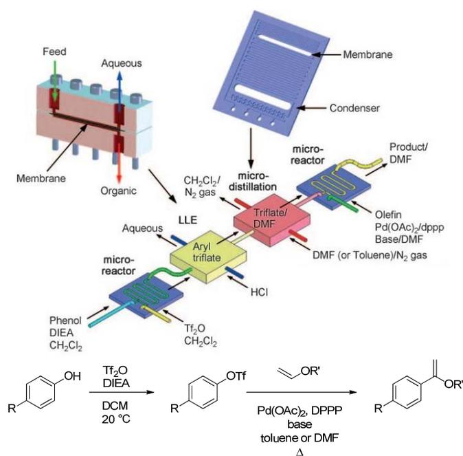
Figure 6. Multistep reaction sequence with liquid-liquid extraction and single stage distillation for solvent switch.<sup>30</sup>
