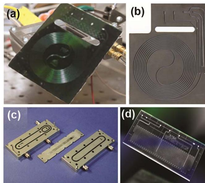
Figure 3. Examples of microstructured reactors in (a) silicon-Pyrex,<sup>20</sup> (b) ceramics,<sup>21</sup> (c) stainless steel (IMM),<sup>16</sup> and (d) glass (Chemtrix).<sup>22</sup>
