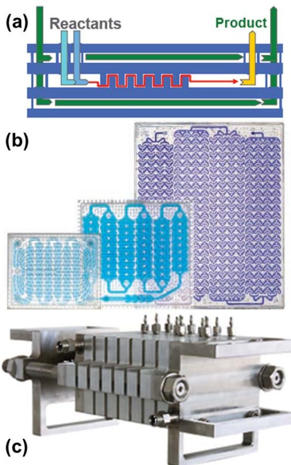
Figure 5. Examples of commercial flow reactor systems for production. (a,b) Corning Advanced Flow Reactors (AFR);<sup>24</sup> (b) Glass reactor plates of increasing size. Note the size of the static mixer structures remain similar with scaling of the plates. (Corning) (c) Lonza flow plate technology<sup>25</sup> in stainless steel. (Ehrfeld Mikrotechnik-BST)
