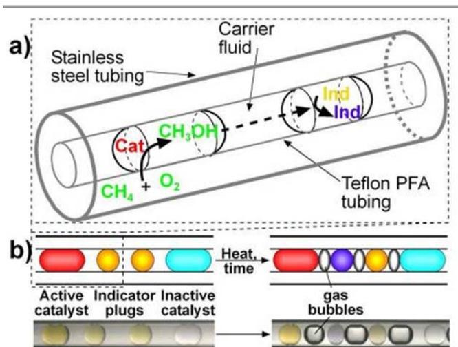
Figure 7. (a) Schematic of a section of Teflon tubing containing droplets inside stainless steel tubing. (b) Schematics (above) and microphotographs (below) show two indicator separating adjacent catalyst plugs to enable clear identification of active catalysts.<sup>41</sup>
