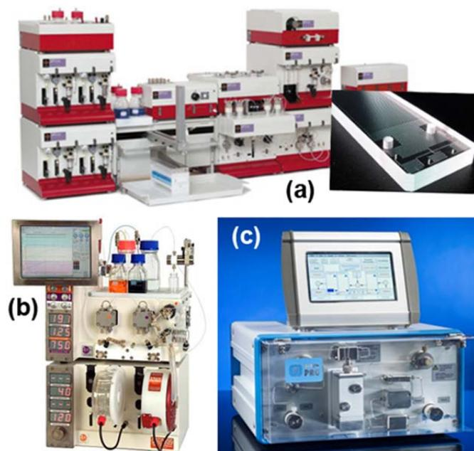
Figure 2. Examples of commercial systems using microreactors and tubes, (a) Syrris Africa system, (b) Vapourtec for general purpose flow chemistry, (c) ThalesNano H-Cube for catalytic hydrogenation.
