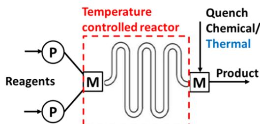
Figure 1. Elements of a continuous flow system. P: Pump; M: Mixer
