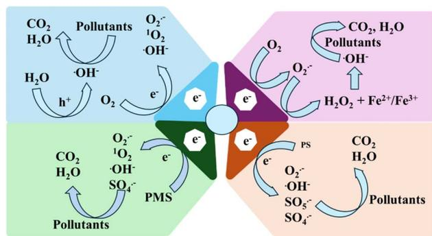
Fig. 11 Generalized wastewater degradation mechanisms using cellulose-supported photocatalysts.
