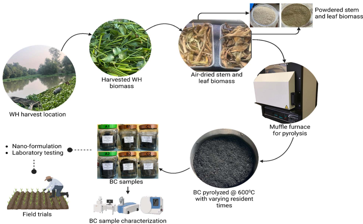
Fig. 1 Process summary for WH upcycling to produce BC for nano-enabled biofertilizer formulation.
