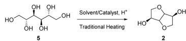
Fig. 10 Isomannide synthesis starting from mannitol, using different solvent–catalyst systems and traditional heating. 20
